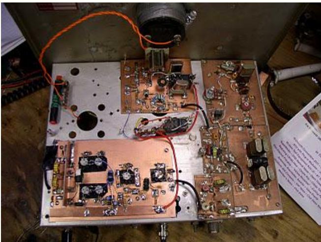
Going around, clockwise from below the meter: G3RJV VXO, carrier oscillator and two diode balanced modulator board, crystal filter (with NE602 mixer and post-filter bandpass filter to the left), JBOT PA. Audio amp (using
